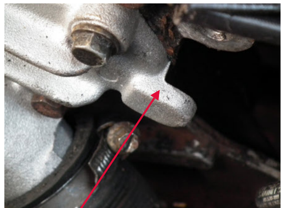
6. This lug needs to be cut off. Easier on bench before you fit pump.
