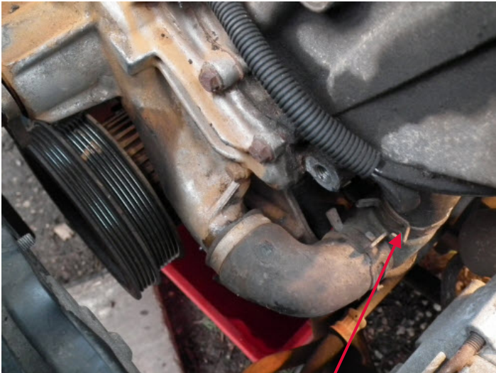
1. Here is what we start with. This is external Thermostat
