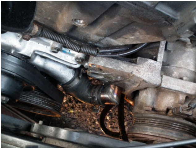
9. Bracket and pump back on. Just belts etc to put back on. Make sure these pipes are not rubbing on the radiator hose
