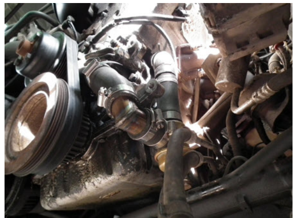
Fitted in place, bottom hose yet to be fitted after replacing radiator.
